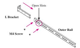
Secure L Bracket to outer rail with 1 or 2 M4 screws. Do not tighten yet. 2
